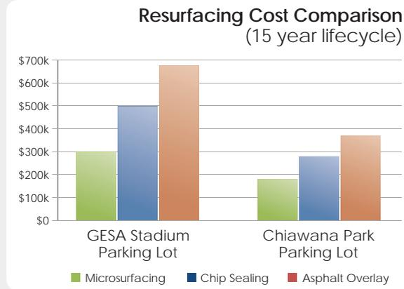
the cost savings are significant (microsurfacing costs as little as 20% of the cost of an overlay). While microsurfacing is typically done every 7-8 years (as compared to every 12-15 years for an overlay) the process extends the life of asphalt significantly, resulting in savings of more than 60% over the useful life of the pavement.
